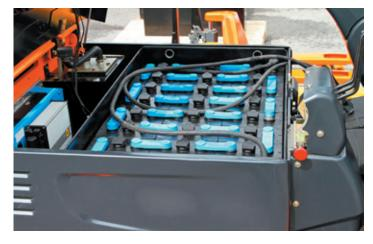
A minimal amount of attention is paid to batteries while recharging or while in operation. This means developing faults can remain unidentified until the point of failure. Intervention is unlikely and the damage or loss maybe limited only by the combustibility of surrounding materials. For this reason, it is best practice to provide a charging space free of conditions that would allow the development of an explosive atmosphere or development and escape of fire beyond the appliance.
