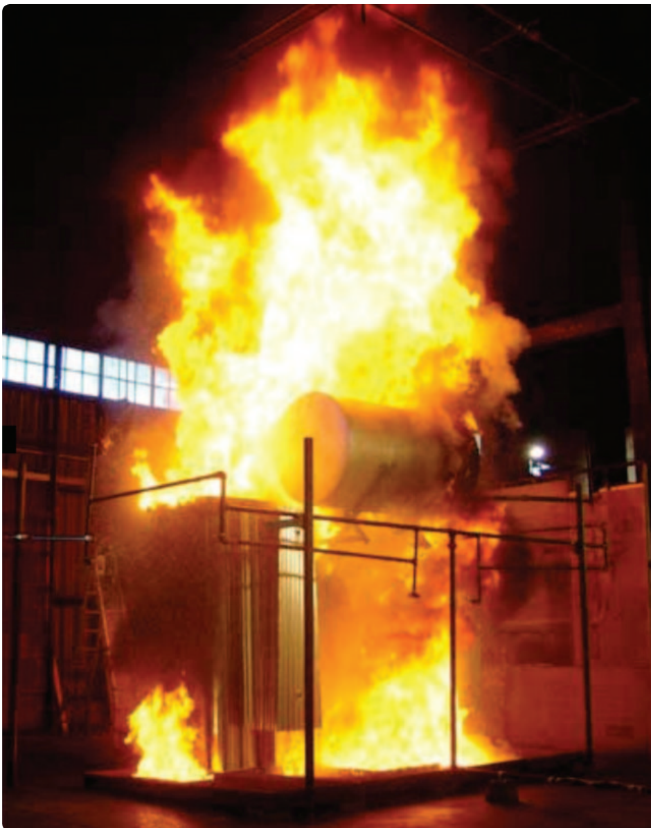
Figure 2: Oil Filled Transformer Fire (Source NRC Canada)
