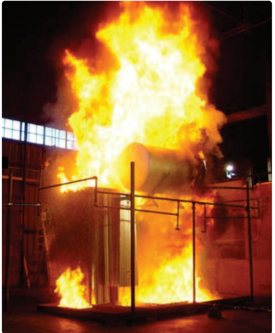
Figure 3: Oil Filled Transformer Fire (Source NRC Canada)
