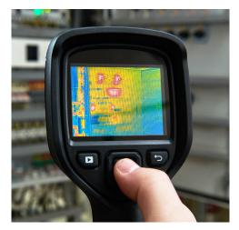
While ITS is quite often used for detecting electrical abnormalities it can also be used as a condition monitoring tool for electrical motors and mechanical bearings.
