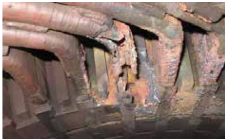
Figure 2: Large motor stator winding insulation failure. Photo courtesy of Machinemonitor Pty Ltd
